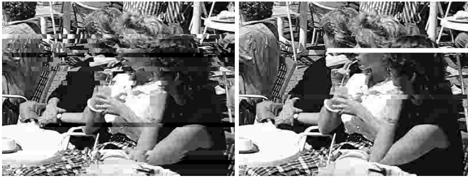
Fig. 15. Magnified portion of the "cafe" image coded with JPEG at 0.5 bpp, when transmitted over a channel with bit error rates of 10^{-4} (left) and 10^{-5} (right). The images shown are the ones with median MSE, of 200 runs.
