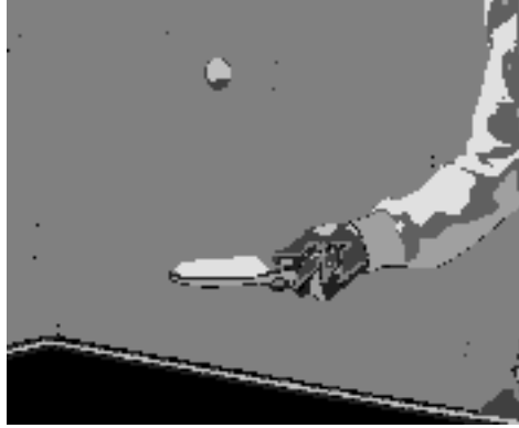
Figure 17: an example of a segmentation obtained by vector quantization with 8 regions (i.e. codebook size of 8).
