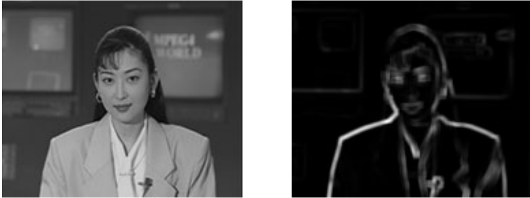
Figure 7: original image (left) and its local variance, var (right), over a 5 \times 5 window.
